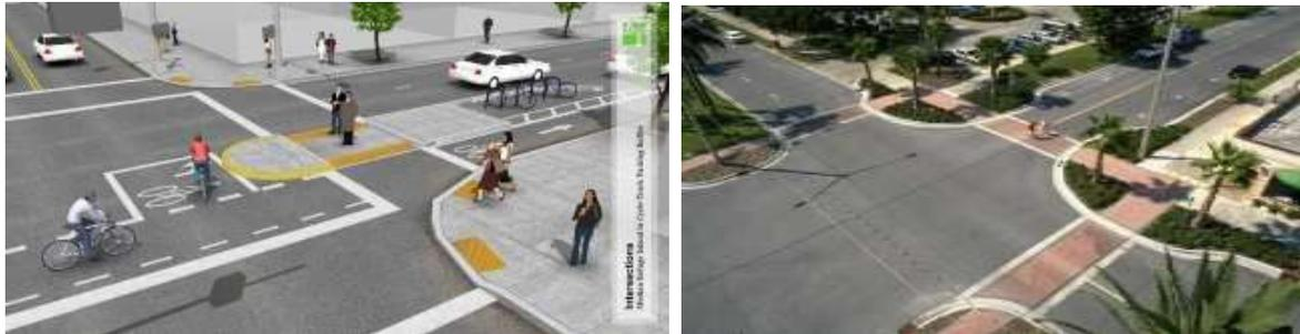
Figure 2: Median islands and curb extensions are two examples of traffic calming measures.
